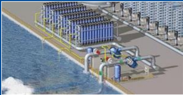
seawater desalination (RO)
